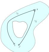
A topological feature of the configuration space inducing instability on the motion planning.
